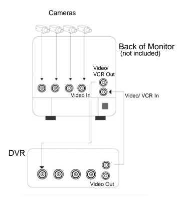
A quad monitor without looping video outputs for each channel should have a video output labeled VCR out
